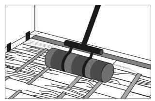
• Use 45-70kg roller to apply pressure to installed sections while the adhesive is still active (approximately 45-60 mins).
